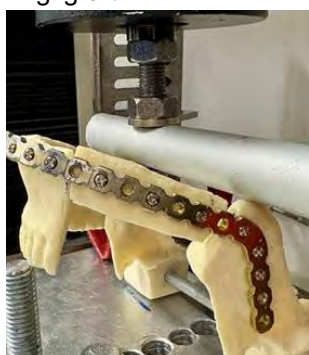
Figure 3: Mandibular reconstruction model with a high-profile plate and fibula-simulating graft positioned for biomechanical testing
